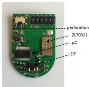
**Image 3** System board with microcontroller, radio module and connectors to sensor chip, antenna and programming device; the latter is cut-off prior to integration along the perforation line; width of the device is 27 mm.
