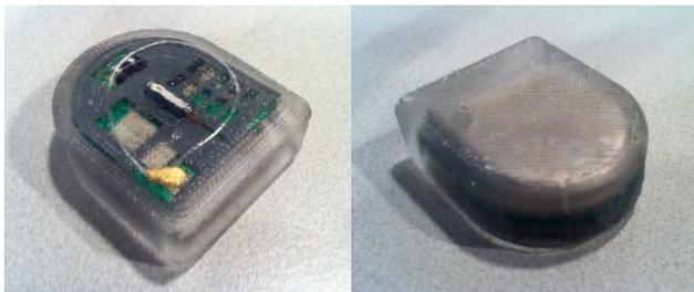
**Image 5** Silicone-encapsulated glucose monitor implant from **left** top-front and **right** bottom-rear perspectives; dimensions of the device are  $38.6 \times 49.3 \times 15.5$  mm [26].
