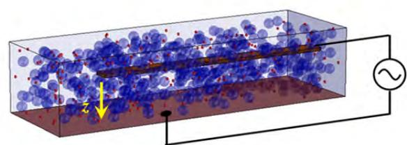
**Image 1** Principle of affinity viscosimetry based on a microelectromechanical system (MEMS), see [8].
