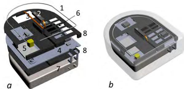
**Image 4 a** Explosion scheme of the sensor implant encompassing the antenna 1, sensor probe 2, flex cable 3, system board 4 with frontend chip 5 and microcontroller 6, battery 7 and distance holders 8. **b** Implant design as integrated in a transparent silicon housing.
