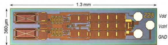
**Image 2** Sensor chip with fully embedded BioMEMS [8].
