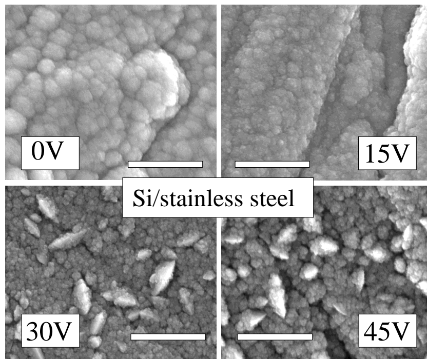
Fig. 3. Top-view SEM micrographs of silicon films deposited on stainless-steel substrates at different susceptor biases V_S (0, 15, 30, and 45 V). The bars are 1 \mu\text{m} long.
